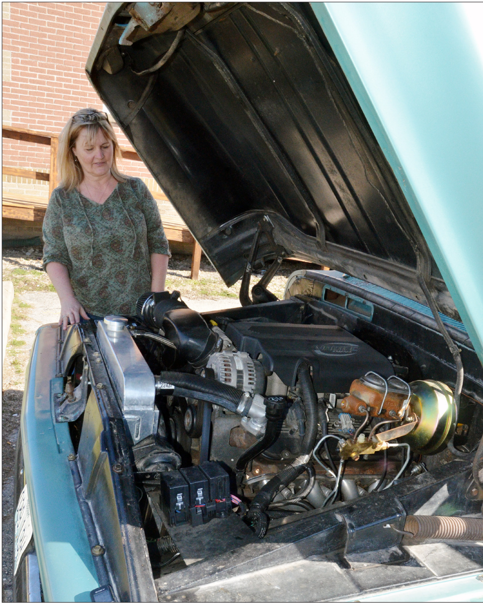
THE 8.1L big block V8 (above) from a 2002 Chevrolet Suburban was a little larger than the engine compartment of the '65 C10. So some adjustments had to be made. The Wrights still need a bumper for their truck (right).
