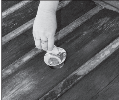
THE GAS cap is accessed in the truck bed with a special tool.
