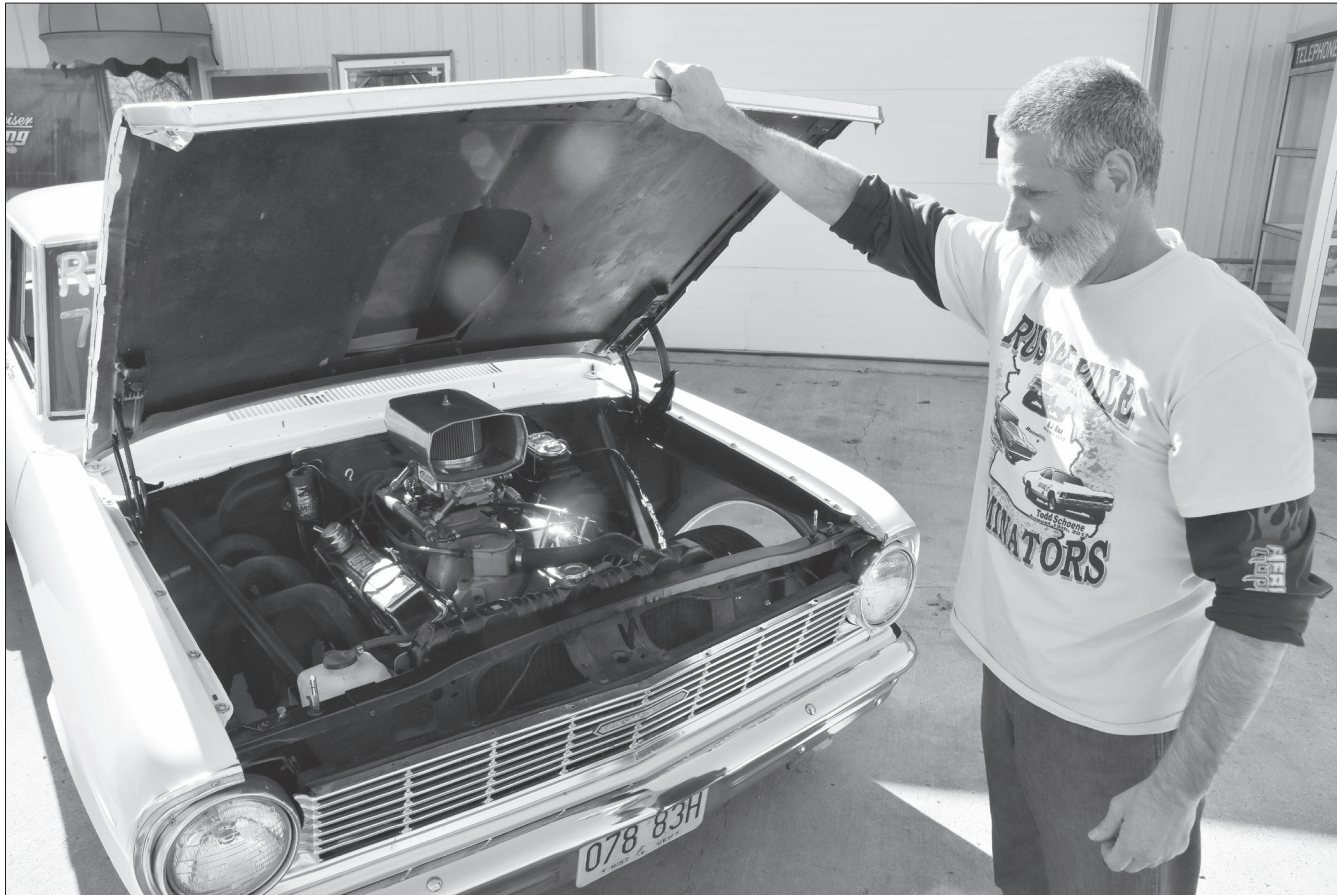
THE 1965 CHEVY has a 540 cubic inch big block V8 engine that runs on alcohol producing 814 horse power.
