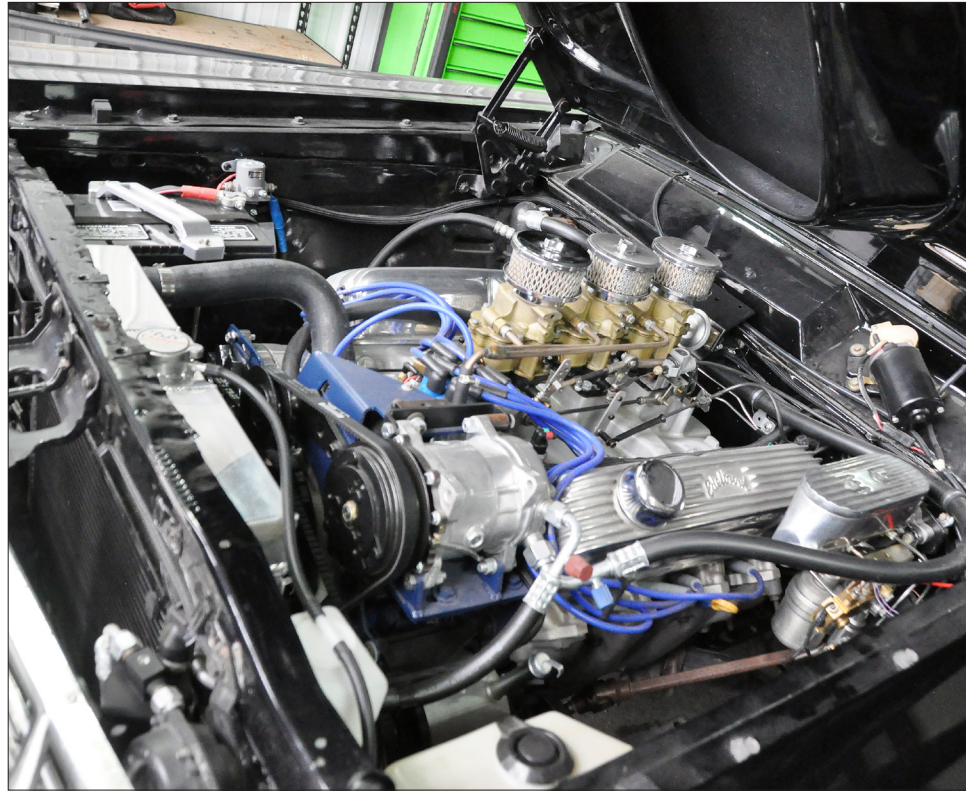
THE '67 Fairlane has a 390 cubic inch V6 board 40 over with a six-pack intake manifold.
