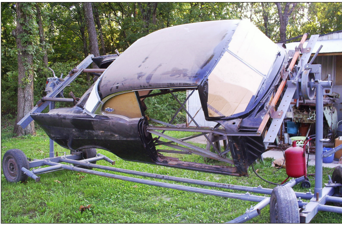
DORTON BUILT a custom rotisserie (photo left) for his 10-year project to restore the wrecked 1957 Chevrolet Bel Air he purchased from Mike Riefer in 2006. The wreck, in April 1982, required that he replace the front quarter panels and the engine compartment (photo right). Dorton worked on the car three to five night each week from 2010 to 2021.
